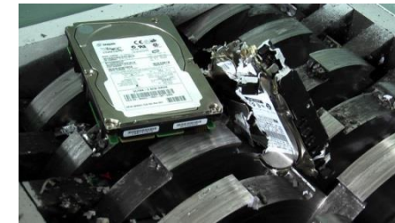
Granulator cutting cylinder
